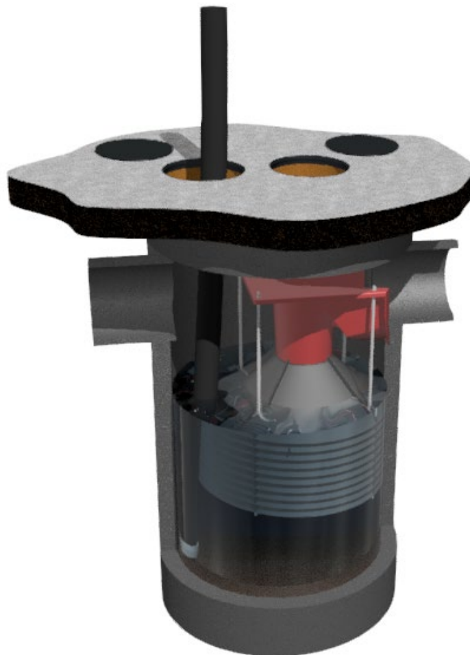
Fig.4 Floatables are removed with a vactor hose
